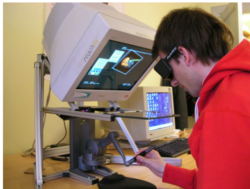
Fig. 1. The Reachin desktop display [10]. The PHANToM device [11] is positioned beneath a semi-transparent mirror. The graphics are projected through the mirror to obtain co-location of graphics and haptics.
